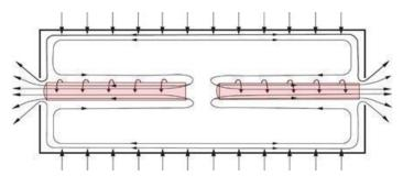
Gas flow pattern inside ASP separation device.
