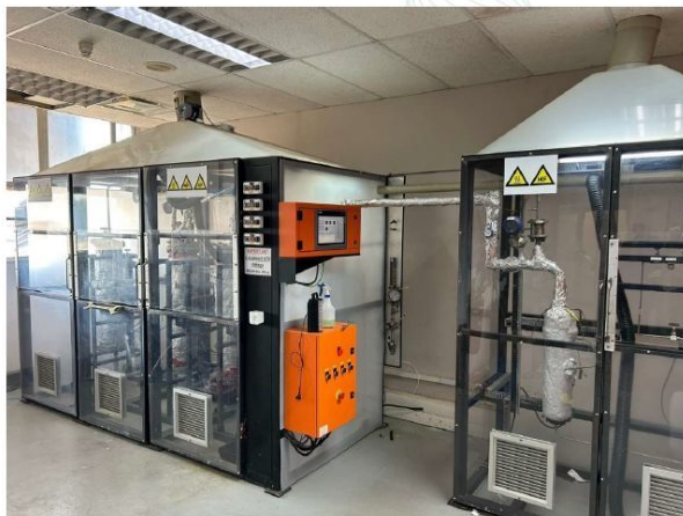
Pilot plant capable of producing 220 tons per annum of fluorinated rare earth metals.
